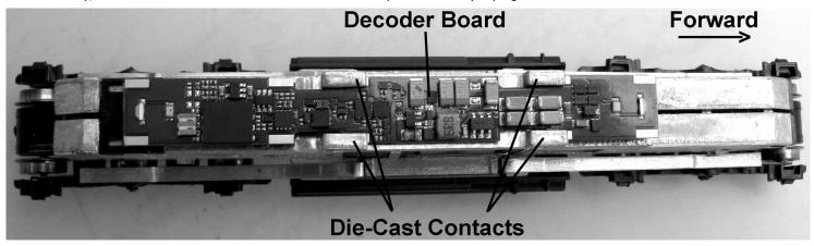
There are no user serviceable parts on the decoder. If it should fail for any reason, it will have to be returned to InterMountain for replacement. Contact us for more information should you need a replacement decoder.
