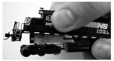
Once the shell is off you will see the decoder on top of the die-cast chassis. If you need to remove the decoder for any reason, sliding it forward gently will release it from the die-cast contacts. The decoder can only be installed one way so if it doesn't slide back in easily, don't force it. Check that it is oriented correctly and carefully try again.
