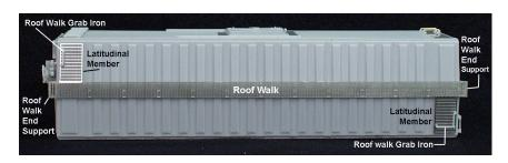
Step 19. Attach the roof walk grab irons to the latitudinal members, and the roof walk end supports in the locator holes provided at the top of the end. Enlarge the locator holes for the roof walk end supports with a no. 70 (.028 in. dia.) drill. The body assembly can be painted now.
