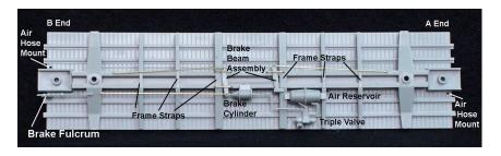
Step 2. Remove the six frame straps from their sprue. Attach the one wide strap which has a small hole in the recess at the wide center cross bearer that also has a small hole. Attach the other wide strap and the four narrow straps into the other recessed locators between the cross bearers of the frame.
