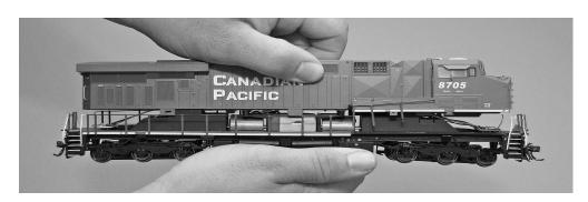
2. To remove the shell, firmly grip the fuel tank area and the center area of the body. Gently rock the shell side to side to release the holding tabs and lift straight up. Watch that the handrails do not get caught on the body deck or cab while being lifted off.
