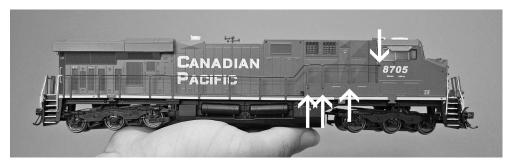
1. The handrail is attached to the cab and deck that need to be removed. Loosen the stanchions (vertical posts) from their attached positions, note the first four stanchions on the left side (not shown) also need to be removed along with the first three on the right side (shown above). Remove the handrails from the nose of the locomotive as indicated in the image to the right.
