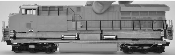
**3.** The shell should slide off of the chassis to reveal the mechanism and electronics. There are no wires attaching the shell to the drive.
