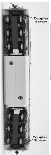
**2.** Pull upward on the shell using a steady controlled pressure. Be gentle and take your time to avoid damaging any of the locomotive details. Once the die-cast chassis begins to slide out from the shell, take care to guide the front and rear portions evenly. <u>DO NOT wedge the chassis against the shell.</u>
