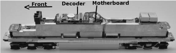
**4.** To reassemble the locomotive, place the shell over the drive mechanism and gently press downward and evenly until the shell snaps into place. Slide the front and rear coupler boxes (with couplers) back into place and replace the screws.
