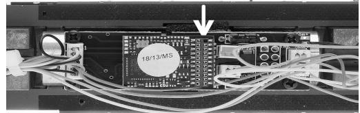
2. After the decoder is removed, install the 21-Pin DC Circuit Board plug onto the pins. Note that the black header faces UP! The pins and plug are keyed to assist the correct installation. Be sure to fully seat the DC plug straight onto the pins without bending them.
