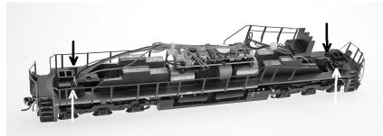
Once you have the body off you will have full access to the circuit board, speaker (sound units only), trucks, and light circuits. If you need to remove the skirt deck, remove the four (4) screws holding in the light boards (as indicated by the arrows). The light boards will then release the skirt to be lifted off the frame.
