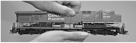
To remove the shell, firmly grip the fuel tank area and the center area of the body. Gently rock the shell side to side to release the holding tabs and lift straight up. Watch that the handrails do not get caught on the body deck or cab while being lifted off.
