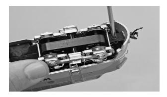
1. Place the locomotive on a soft surface or foam cradle. Remove the front coupler from the locomotive. Utilize a Philips head screw driver to unscrew the coupler from the frame. Gently slide the coupler box from the shell and frame. The coupler box may need to be disassembled in place and removed as separate pieces. Keep the pieces together for re-assembly.
